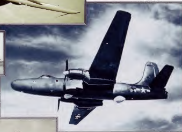
▲ Designed for speed and range Like the Consolidated PB4Y before it, the P4M used a long, thin wing to provide fuel capacity and long range. The jet engines, while providing more speed, actually compromised range performance.
